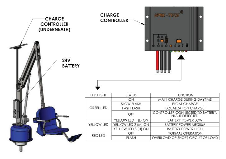
Once the solar charger has been installed and plugged into the control box, and there is sufficient daylight, the 24V Solar Charger will turn on and start trickle-charging the battery.
