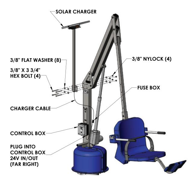
The 24V Solar Charger bolts directly to the mast of the lift and may be left on the unit 24 hours a day. In most cases this will mean the battery will not need to be charged during the day, or for heavy usage will not need to be put on the AC wall charger as often. To install the 24V Solar Charger, remove the four (4) 3/8" Nylock nuts and flat washers from the lift as shown, and install the charger. The control box connector plugs directly into the control box as shown above and on page 3.
