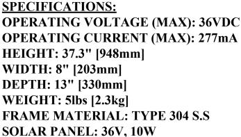
**CHARGE CONTROLLER: PROTECTION RATING: IP68** [CONTROLLER: 1.5m 72 HOURS] SHORT CIRCUIT PROTECTION **REVERSE POLARITY DETECTION OVERCHARGE DETECTION** (PREVENTS BATTERY DAMAGE)
