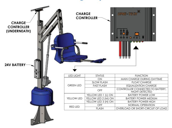
Once the solar charger has been installed and plugged into the control box, and there is sufficient daylight, the 24V Solar Charger will turn on and start trickle-charging the battery.
