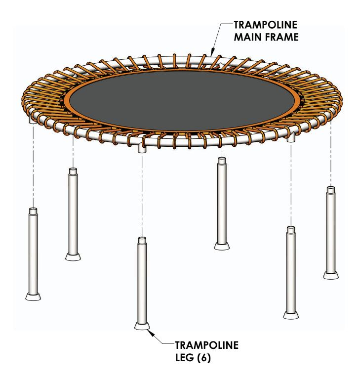
The round trampoline will come with the six (6) legs unattached. To attach, simply thread the legs into the six (6) leg locations welded onto the main frame of the trampoline. See image above.
