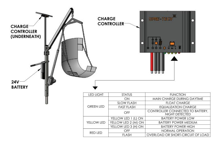
Once the solar charger has been installed and plugged into the control box, and there is sufficient daylight, the 24V Solar Charger will turn on and start trickle-charging the battery.
